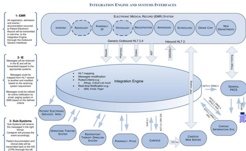
**Figure 3.** The main components of the EMR system at NGHHA showing the integration engine used to integrate the different clinical systems.....
